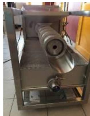
Make sure that no material other than the uncapped wax is filled into the filling opening. The percentage of the honey extracted from the wax, i.e. the efficiency of honey extraction reduces with the increase of the applied rotations. Optimal rotations: 30-70% of the maximum rotations.
