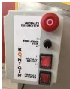
Turn on the main switch on the plug to energise the machine. It is important to check the red emergency button for its condition. It must not be pressed. Otherwise pull out or turn the emergency button to inactivate the emergency status.
